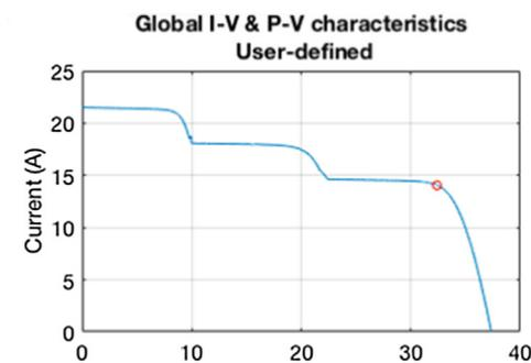
(b) I-V and P-V characteristic before reconfiguration ( $P_{MPP} = 456W$ )
