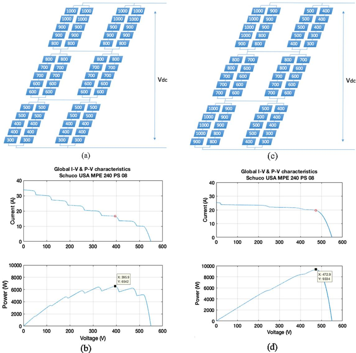
Fig. 15. Diagram comparing the output power of the solar power system with (a) the reconfiguration system  $P_{max} = 9334$  W and without (b) reconfiguration system  $P_{max} = 6542$  W when in PS situations.
