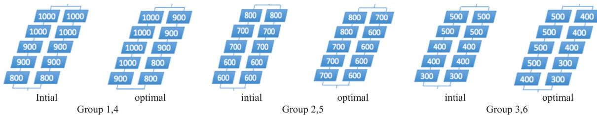
Fig. 16. Initial and Optimal configuration of each group in SP topology.
