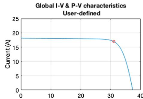
(d) I-V and P-V characteristic after reconfiguration ( $P_{MPP} = 526.9W$ )
