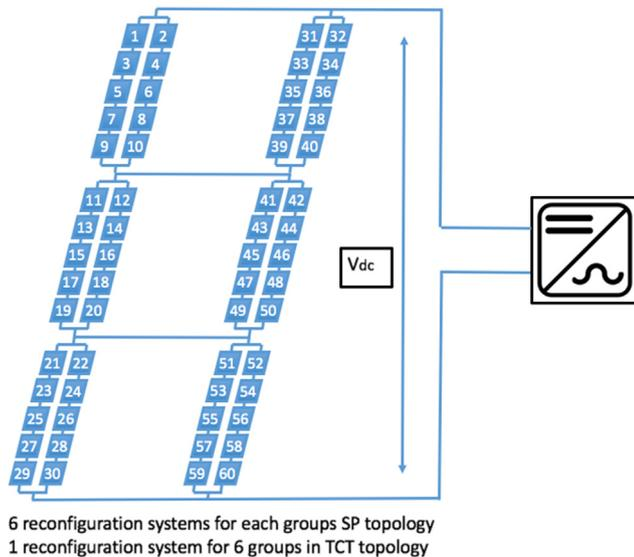
Fig. 13. Subgroup design diagram of PV system.
