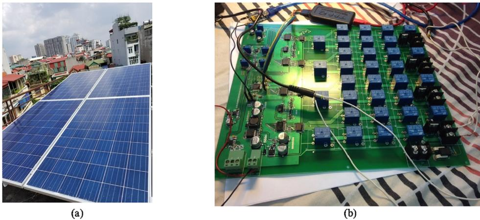
Fig. 8. PV system with reconfigurator: (a) PV panels; (b) Switching matrix for SP topology.
