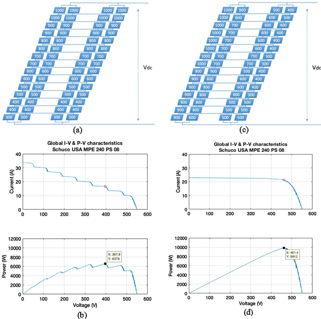
Fig. 19. Diagram comparing the output power of the solar power system with fully controllable Switching matrix in TCT topology.
