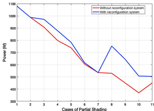
Fig. 11. Diagram comparing the output power of the solar power system with the reconfiguration system and without reconfiguration system when in partial shading situations.
