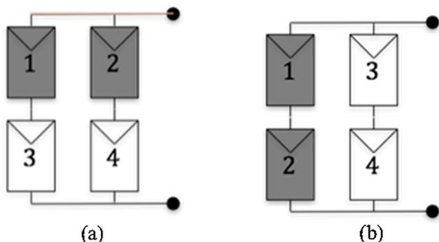
Fig. 9. Connection of PV system before (a) and after (b) reconfiguration.
