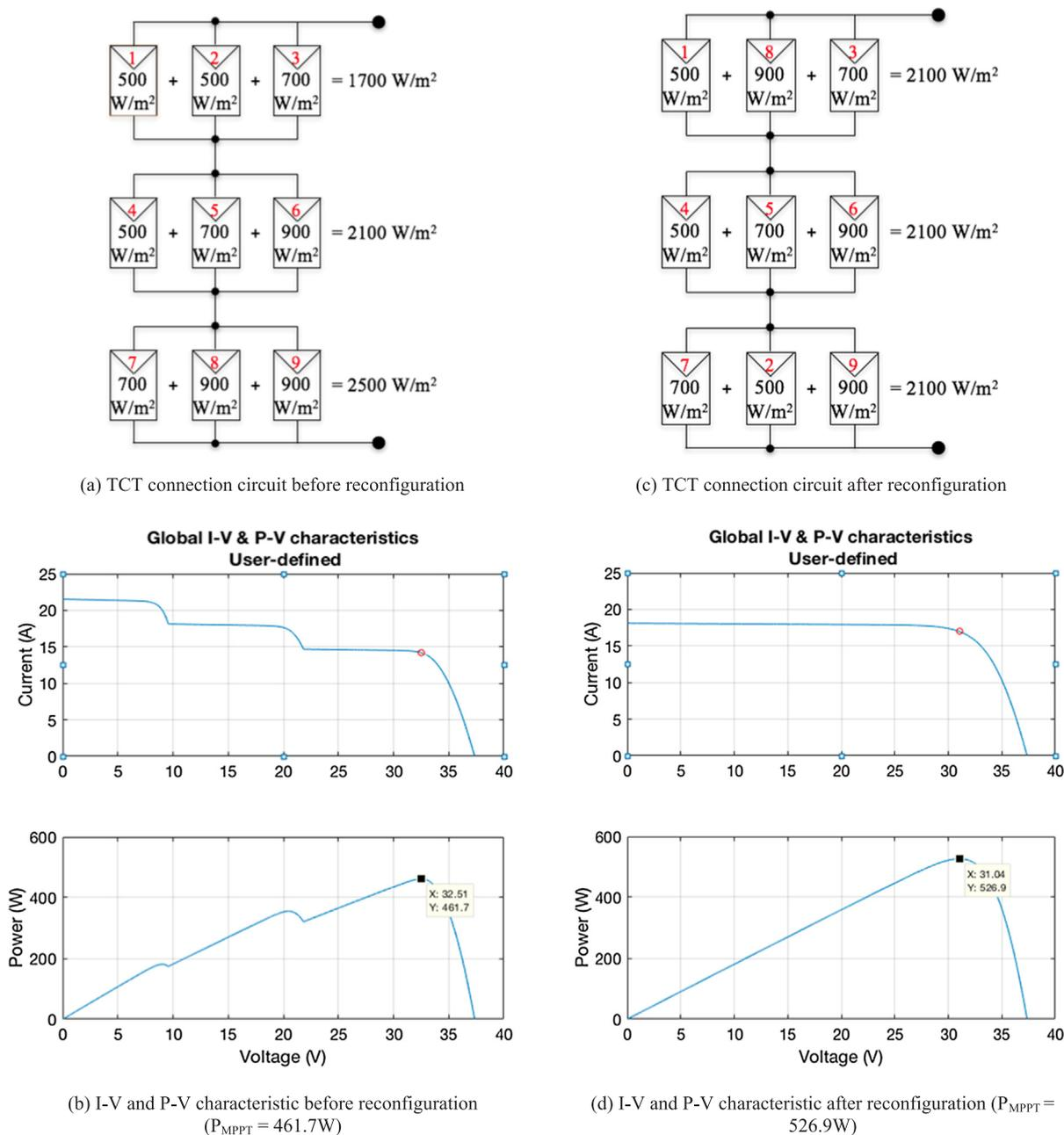
Fig. 2. PV system (a) and I-V P-V characteristic (b) before reconfiguration; PV system (c) and I-V P-V characteristic (d) after reconfiguration.
