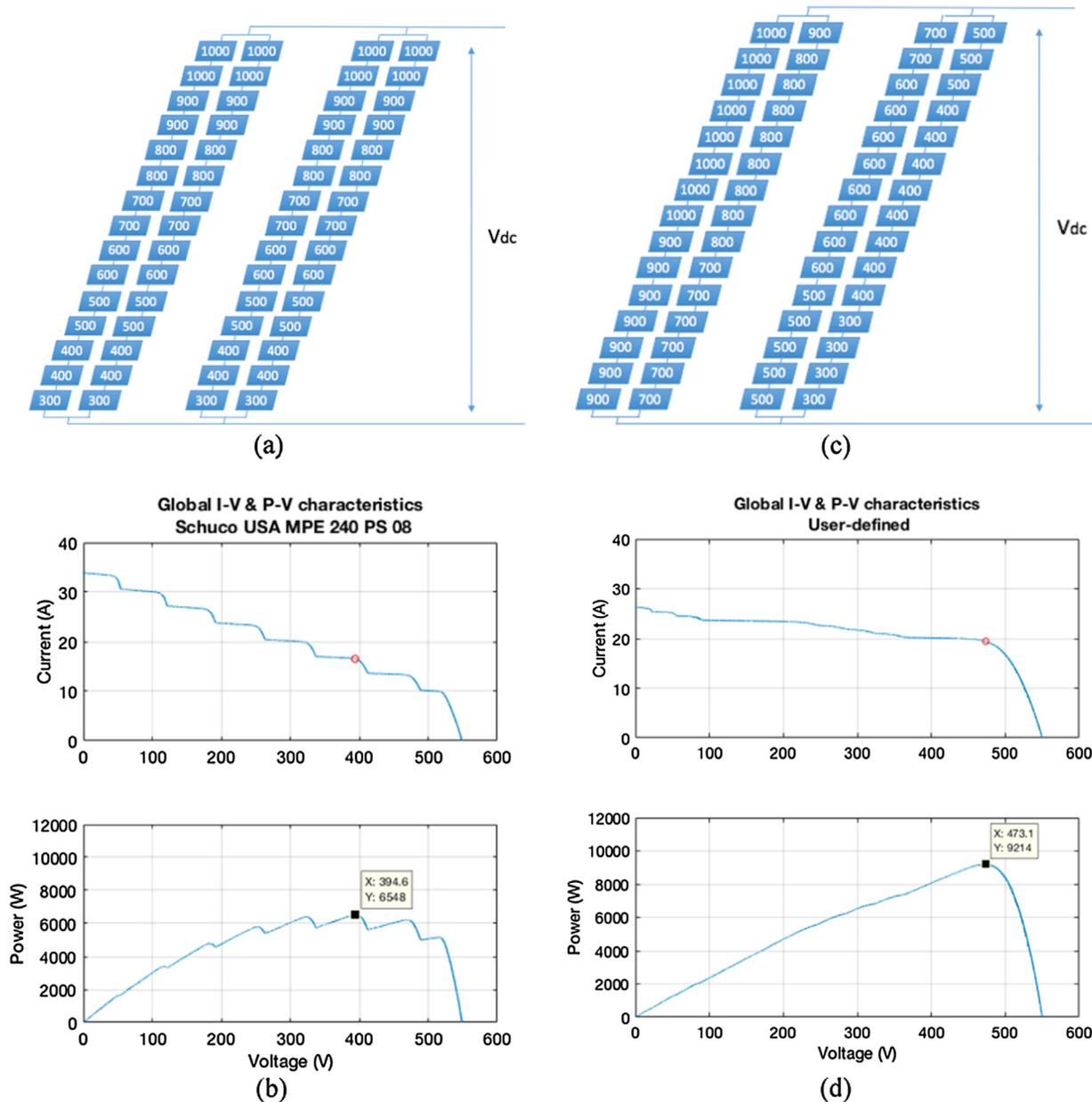
Fig. 18. Diagram comparing the output power of the solar power system with fully controllable Switching matrix in SP topology.
