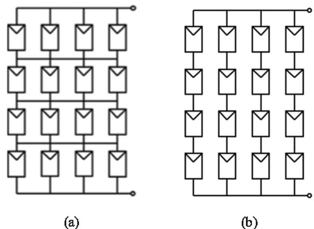
Fig. 1. Connection topologies of the PV array (a) Total-cross-tied topology (b) Series-Parallel.
