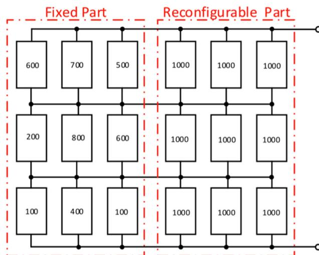
Fig. 12. One situation in which the system proposed in Tubniyom et al. (2019) would not work (partial shading only on Fixed Part).
