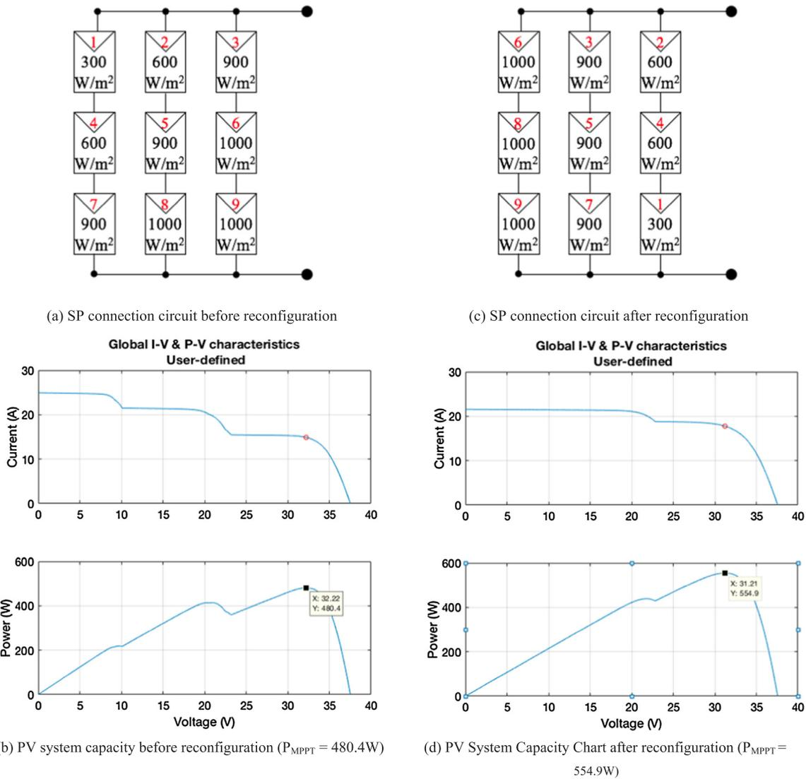
Fig. 7. Simulation of the numerical example of the methodology for enhancing the efficiency of the SP connected PV plant, (a, b) show the original system with the  $P_{MPPT} = 480.4\text{ W}$ , (c, d) after reconfiguration with the  $P_{MPPT} = 554.9\text{ W}$ .
